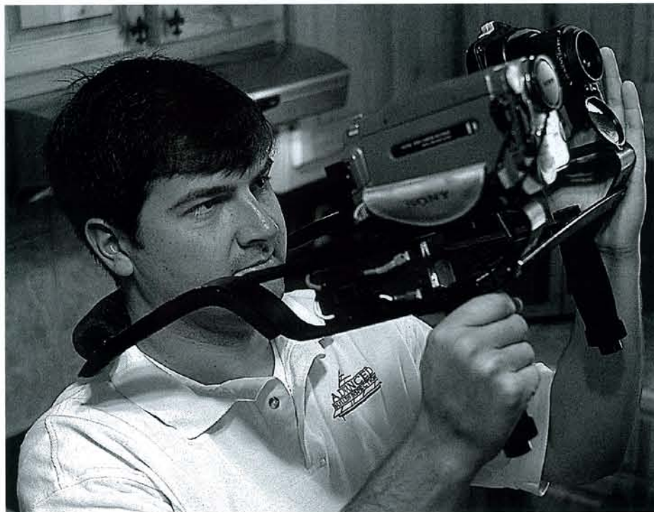
NO SUPERMAN: It's not quite X-Ray vision, but Spencer Maxcy's infrared equipment allows him to see hidden leaks and termite activity in the homes he inspects. An improperly installed HVAC unit leaks into a stud-and-sheetrock wall, but only the IR image (below right) can see it.
